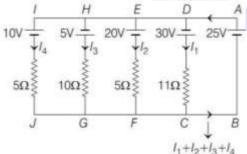
Applying KVL in closed loop ADCBA, AEFBA, AHGBA and AIJBA, we get  $30-11I_1+25=0$   $-20-5I_2+25=0$   $5-10I_3+25=0$   $-10-5I_4+25=0$ From Eqs. (i), (ii), (iii), (iv), we get  $I_1=5A, I_2=1A, I_3=3A, I_4=3A$  $I=I_1+I_2+I_3+I_4=12A$
